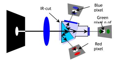
Fig. 9. 3 CCD prism construction.
